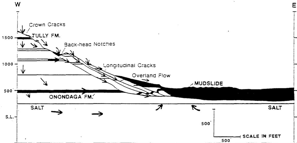
Figure 5. Cross section showing possible groundwater migration routes.
